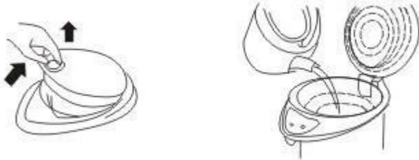
Press the lid opening switch to unlock the lid's top cover and open it.
